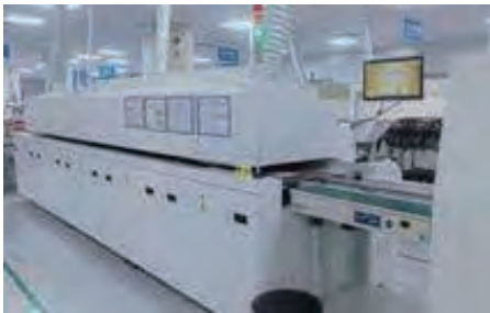
Automatic Reflow Machine
