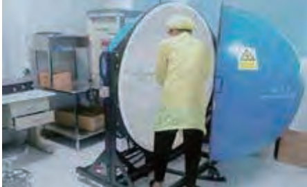
The FAI test ,to make sure the electric-optical characteristics is correct.
